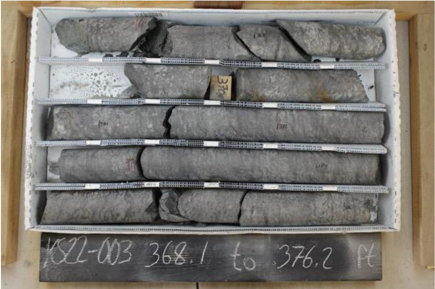
KS22-003 Core photo of magnetite rich ultramafic with nickel sulfide
